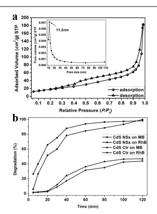
**Fig. 3** (a) Nitrogen adsorption/desorption isotherm of the CdS NSs, inset: the corresponding BJH pore size distribution curve. (b) Photocatalytic degradation of RhB and MB in the presence of the CdS NSs and CdS Ctr under visible light irradiation.
