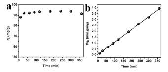
**Fig. 4** (a) The adsorption curve of the CdS NSs on CR with different adsorption time. (b) Plot of pseudo-second-order kinetics.
