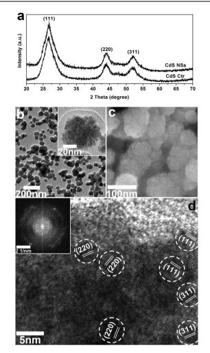
**Fig. 1** (a) XRD pattern of the CdS NSs and CdS Ctr; (b) TEM image of the CdS NSs, inset: high magnified TEM image; (c) FESEM image of the CdS NSs; and (d) HRTEM image of the CdS NSs, inset: SAED pattern of the CdS NSs.
