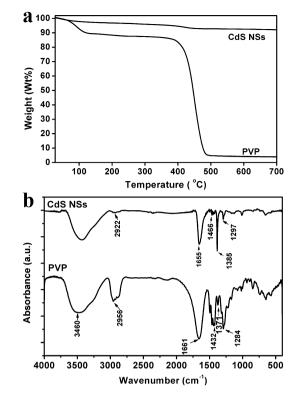
**Fig. 2** (a) TGA curves of the pure PVP and CdS NSs. (b) FT-IR spectra of the pure PVP and CdS NSs.
