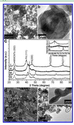
Figure 1. (a) TEM and (b) HRTEM image of the PdCu/MWCNTs. (c) XRD pattern of the PdCu/MWCNTs. Curve I, Pd/MWCNTs; curve II, PdCu/MWCNTs; curve III, Cu/MWCNTs, curve IV, PdCu alloyed nanoparticles. TEM images of samples obtained at (d) 1 h and (e) 3 h; inset, HRTEM image.
