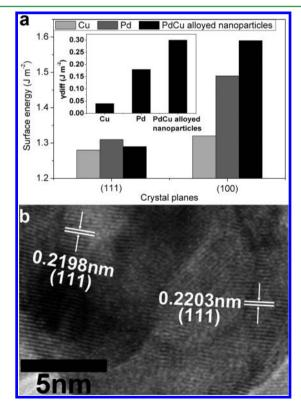
**Figure 2.** (a) Surface energies of the (111) and (100) planes of the Cu, Pd, and PdCu alloyed nanoparticles. Inset: the  $\gamma_{\rm diff}$  between (100) and (111) planes of the Cu, Pd, and PdCu alloyed nanoparticles. (b) HRTEM image of the PdCu/MWCNTs.
