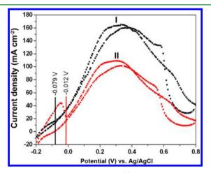
**Figure 4.** Cyclic voltammograms of the (I) PdCu/MWCNTs catalyst, (II) Pd/MWCNTs catalyst in 0.5 M  $\rm H_2SO_4 + 0.5~M~CH_3OH$  aqueous solution.
